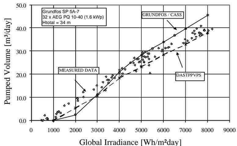
Finally the sizing results of the suppliers have been evaluated. Under real operating conditions, most commissioned systems actually delivered considerably less water than expected.
