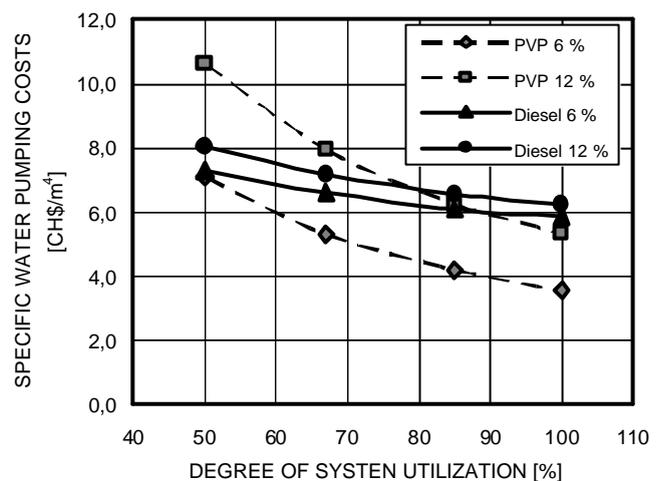
High degrees of system utilisation are necessary to make PVP economically viable. Since the diesel system has a lower investment cost, the water pumping costs react less sensitively to interest rate changes. For low interest rates, the PVP option is economically superior, even at a low rate of system utilisation (50%). At the postulated maximum interest rate of 12%, costs equality is achieved for a utilisation rate of approximately 80%.
