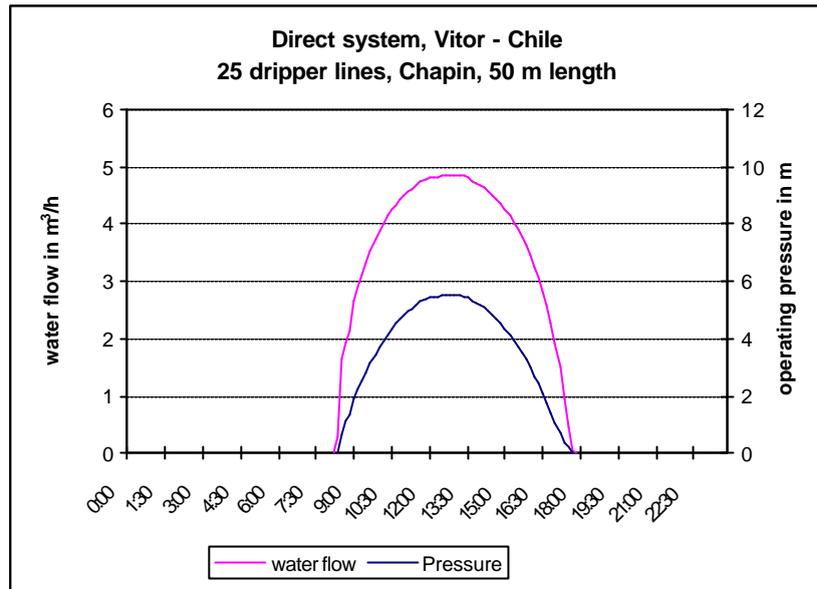
Drip irrigation saves a considerable amount of water compared to other irrigation techniques. Furthermore, it has a rather low operating pressure. Both features reduce the energy demand and make drip irrigation particularly suitable for photovoltaic pumping systems.
