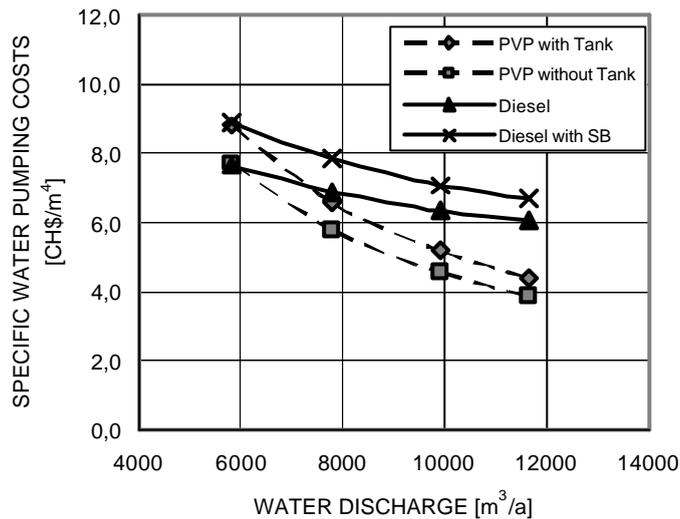
Generally PVP systems tend to be economically viable with a real discount rate below 12% p.a., a degree of system utilisation above 60% and an irrigation area smaller than 4 ha.
